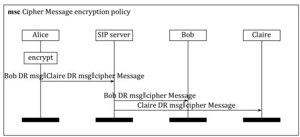
Selection of the encryption policy according to policy parameter, recipientLists and plain text characteristics. The policy parameter is given at runtime by caller and default to *optimize Upload Size* if omitted. Possible values of this parameter are:
